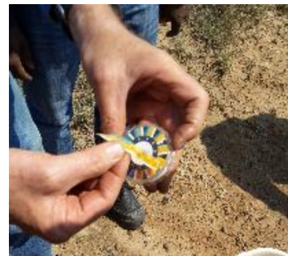
Low soil pH values that, if left unmanaged, can result in significant vegetation die-back
